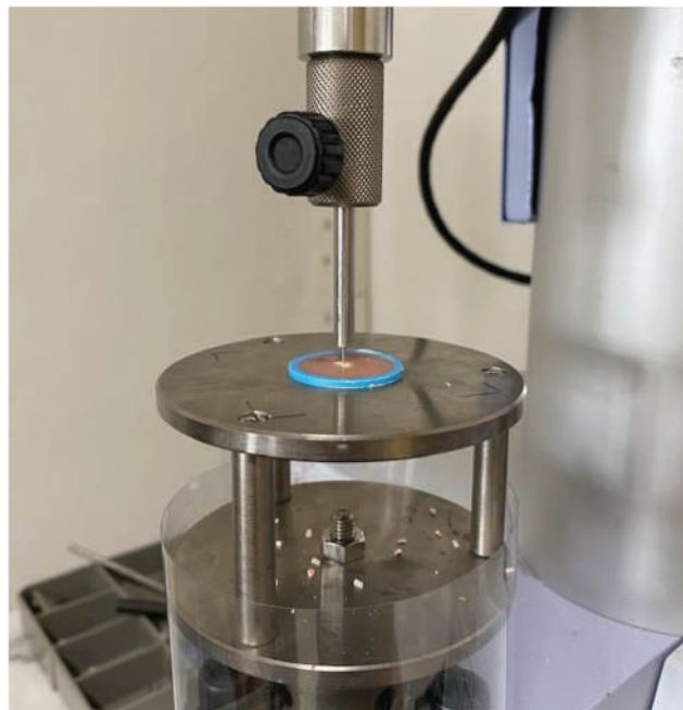
Fig 3. A vertical loading was delivered to the specimen using a Universal Testing Machine.
