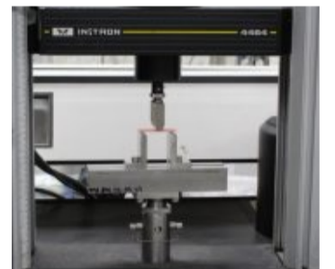
Flexural strength test on instron machine
