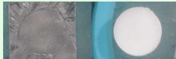
Figure 4: Mixed fracture pattern between titanium-resin cement (RC) (left) and zirconia (Zr)-resin cement (right) interfaces of group TR
