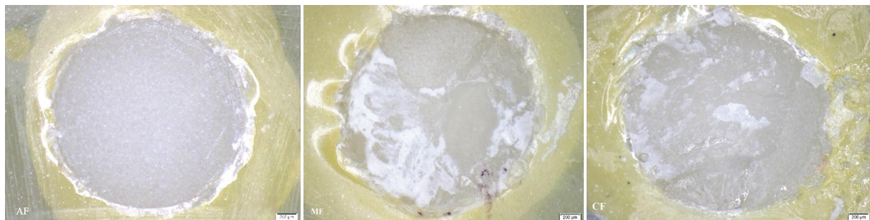
Fig. 5 The stereo microscopic images of adhesive failure (AF) of group 1, mixed failure (MF) of group 6, and cohesive failure (CF) of group 7.
