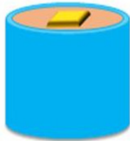
Figure 1. Illustration of specimen embedded in the poly(vinylchloride) tube.
