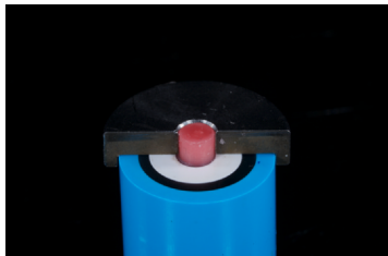
Figure 3. Application of chemically activated chairside hard reline material on CAD-CAM milled PMMA specimen. CAD-CAM, computer-aided design and computer-aided manufacturing; PMMA, polymethyl methacrylate.
