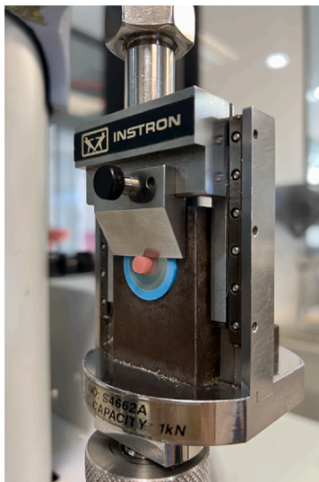
Figure 4. Specimen mounted in universal testing machine for shear bond strength testing.
