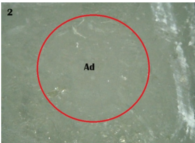
Figure 2. Failure mode of group 1 (Ad, adhesive failure).
